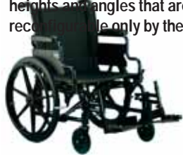
The super-hemi (single-axle) seat-to-floor height is achieved with 22" rear wheels and 6" casters. A 13.5" seat-to-floor height is achieved with 20" rear wheels and 6" casters.
