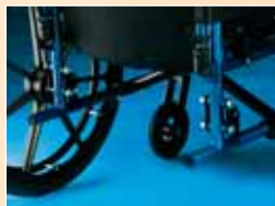
9000XT with offset axle and adjustable angle caster will allow additional seat-to-floor heights and increase seating and positioning capabilities. Offset axle offers center-of-gravity adjustment which increases maneuverability and stability.
