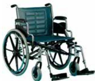
Heavy-duty package increases weight capacity to 450 lb. and consists of heavy-duty composite wheels with pneumatic tires with flat-free inserts and semi-pneumatic casters.
