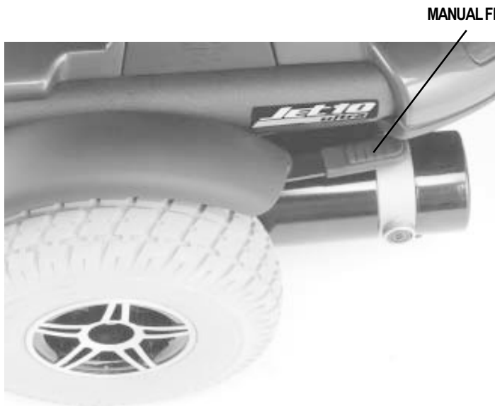
Figure 7. Drive Mode (Drive Engaged)
