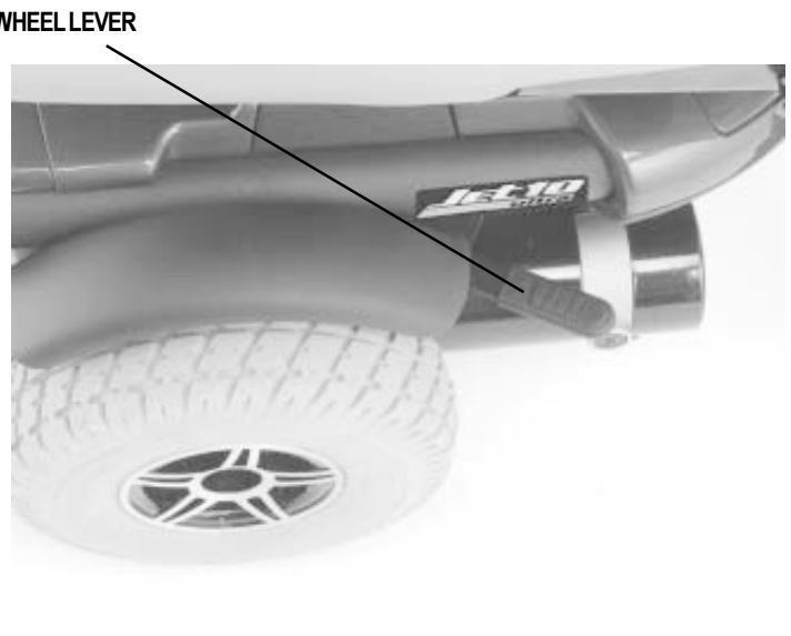
Figure 8. Freewheel Mode (Drive Disengaged)
