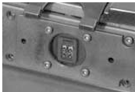
Figure 7. Europa Remote Controller Harness Connector
