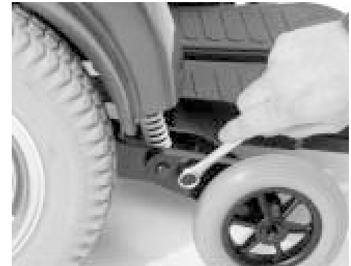
Figure 30. Anti-Tip Wheel Adjustment
