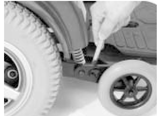
Figure 29. Anti-Tip Wheel Adjustment
