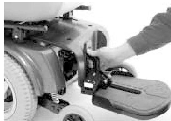
Figure 32. Removing the Foot Frame
