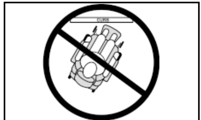
Figure 3. Incorrect Curb Approach
