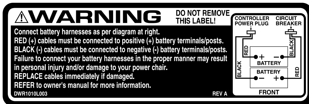
Figure 32. Quantum Jazzy 1420 Battery Wiring Diagram Label
