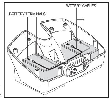
Figure 12. Battery Replacement
