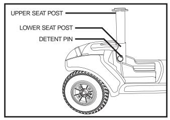
Figure 15. Seat Height Adjustment
