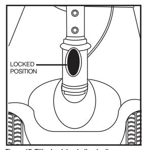
Figure 17. Tiller Lock knob (Locked)
