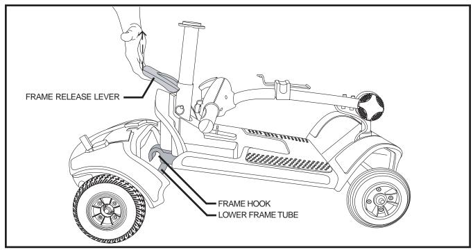
Figure 19. Frame Separation
