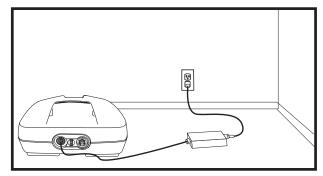
Figure 10. Charging The Batteries (Battery Pack Removed)
