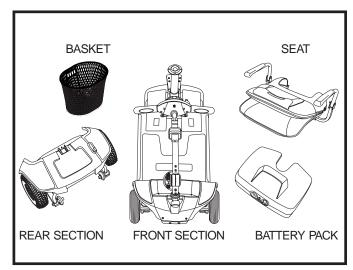
Figure 16. Disassembled Travel Scooter
