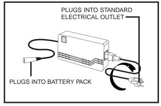
Figure 11. Off-Board Battery Charger
