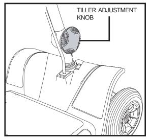
Figure 13. Tiller Adjustment Knob
