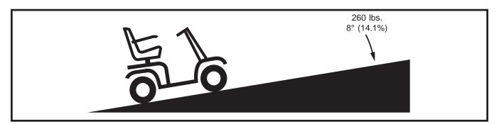
Figure 1. Maximum Recommended Incline Angle
