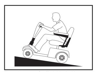
Figure 2A. Increased Stability Driving Position
