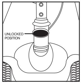
Figure 18. Tiller Lock Knob (Unlocked)
