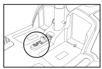
Figure 8. 3-Amp Tiller Console Fuse
