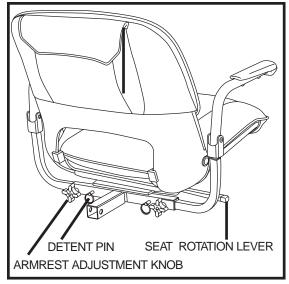
Figure 14. Seat Adjustment
