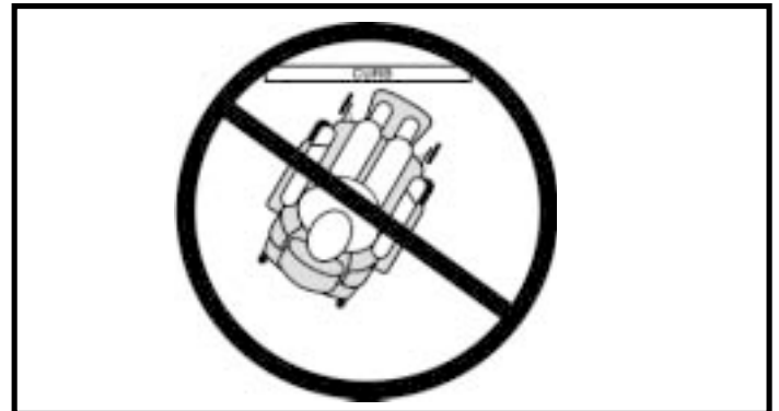
Figure 3. Incorrect Curb Approach
