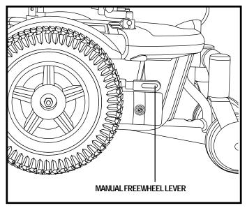
Figure 9. Freewheel Mode (Drive Disengaged)
