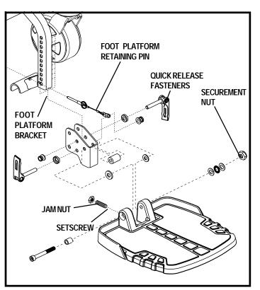
Figure 17. Foot Platform Adjustment
