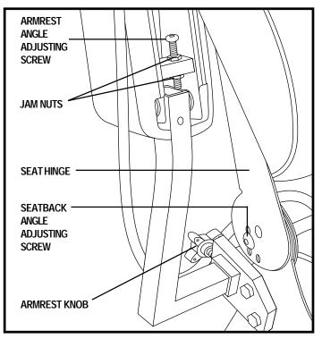
Figure 16. Seatback Angle Adjustment
