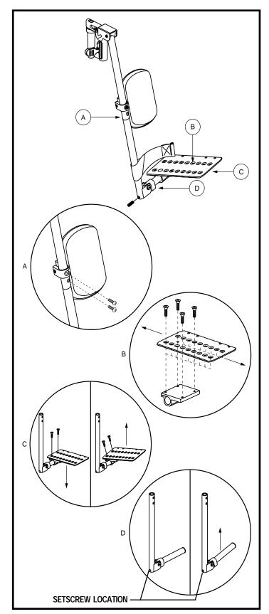
Figure 23. Multi-Axis Foot Plate (ELR Shown)
