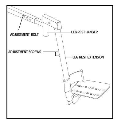
Figure 22. Heavy Duty Drop-In Leg Rests
