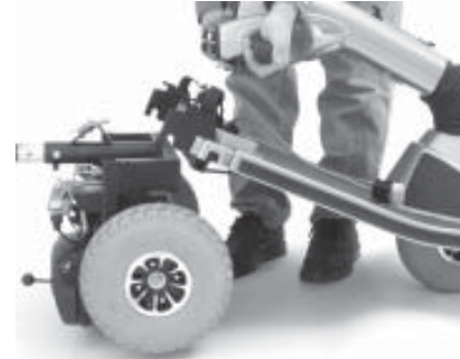
Figure 20. Separating The Frame Sections
