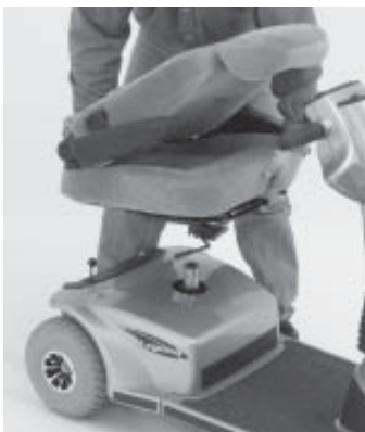
Figure 13. Removing The Seat
