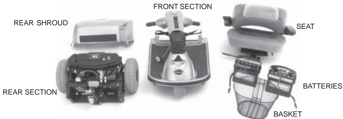
Figure 12. The Legend Disassembled
