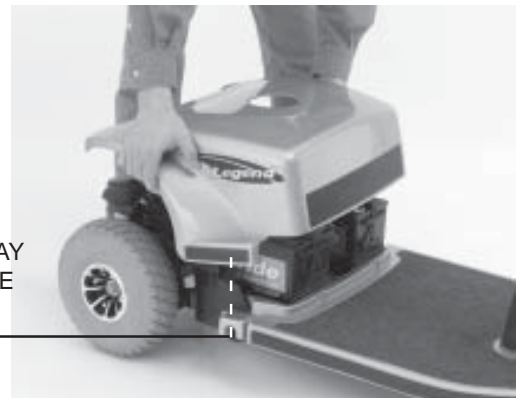
Figure 14. Rear Shroud Removal
