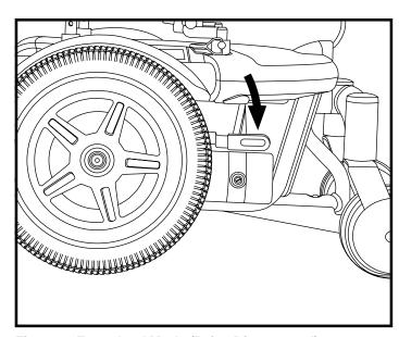
Figure 9. Freewheel Mode (Drive Disengaged)
