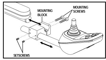
Figure 15. Controller Position - Mounting Block Shown
