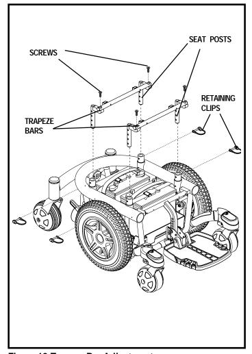
Figure 12. Trapeze Bar Adjustment
