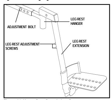
Figure 21. Heavy Duty Drop-In Leg Rests
