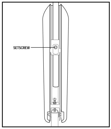
Figure 16. Controller Position - Underside of Armrest
