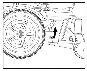
Figure 8. Drive Mode (Drive Engaged)
