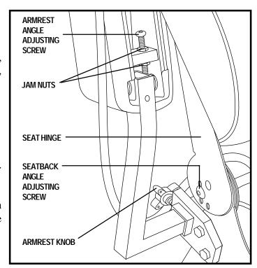
Figure 14. Seatback Angle Adjustment
