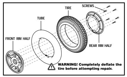
Figure 26. Quantum 600E Drive Wheel Disassembled
