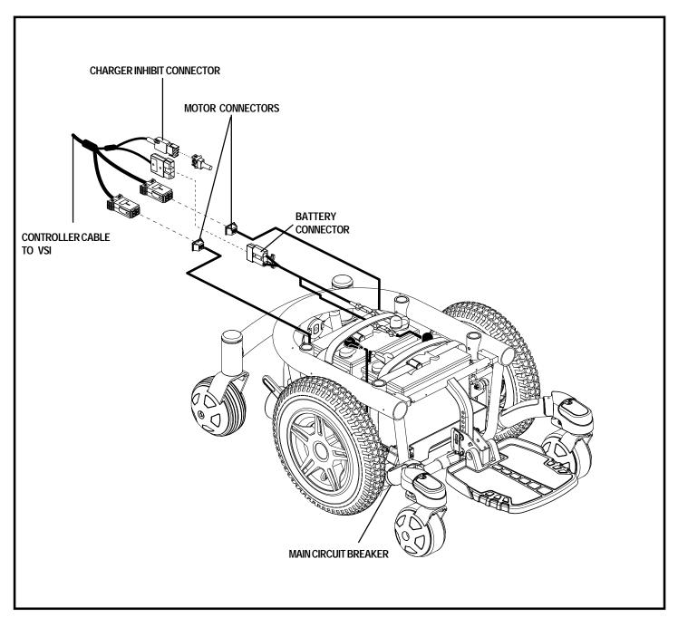
Figure 7. Quantum 600E Electrical Components
